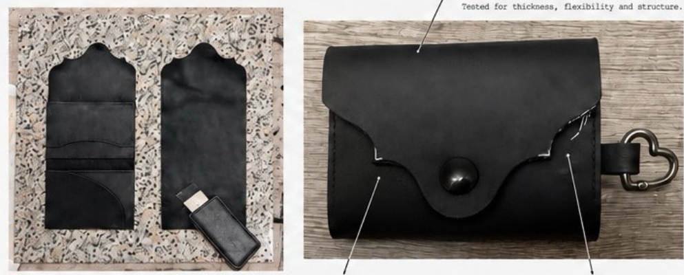
02 FRONT & BACK ASSEMBLY Thinning the sides of the leather pieces before glueing and assemblage.
